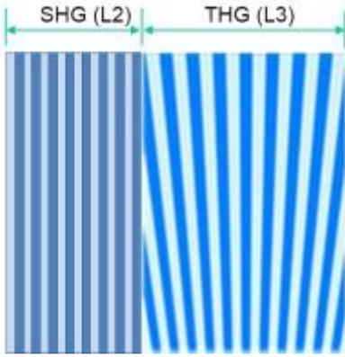
A new robust configuration combined two QPM features: Monolithic and Fan-out structure
