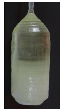
GPS Gadolinium pyro silicate (Ce:Gd 2 Si 2 O 7 )
